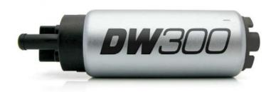
The DW300 is our flagship standard fitment in-tank pump. The DW300 flows 340lph at 40psi and is a popular choice for e85 applications or wherever the highest flowing stanard fitment in-tank pump is needed. Quiet operation and pulse width modulation compatability are delivered via the turbine impeller and computer balanced armature. E85 compatability is built in via the carbon commutators and a fully encapsulated armature. All DW fuel pumps are backed by a 3-yr no fault warranty.
